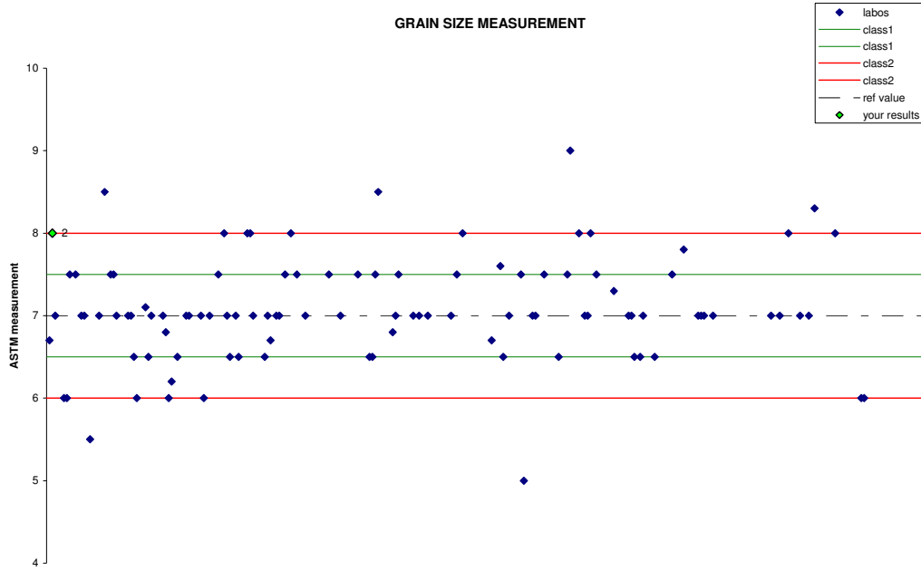
Figure 2 Presentation of grain size results, showing spread of data and limits for classification
